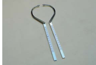
GPM ◀ 102 Recurved measuring branches for anthropometer No. 101 e.g. for measuring sagittal breast diameters
