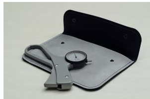
GPM ◀ 6100 «GPM» Skinfold Caliper (made in CH) to assess the degree of fatness measuring range: 0-45 mm
