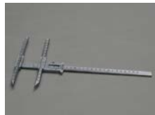
GPM ◀ 115 Coordinate caliper range: 20 -220 mm
