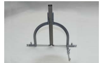
GPM ◀ 122 TODD Head spanner measuring range: 200 mm
