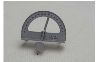
GPM ◀ 117 Goniometer, attachable (Mollison type) range: 0 –180°
