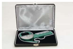
GPM ◀ 120 «LANGE» Skinfold caliper (made in USA) to assess degree of fatness measuring range: 0 – 60 mm
