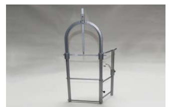
GPM ◀ 208 Combination instruments consisting of: Mollison craniophor No. 209, auricular head spanner No. 210 especially for the adjustment of the skull in the ear-eyes axis 209 / 210 also available separately
