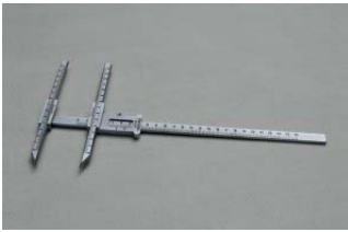
GPM ◀ 114 Sliding caliper (Poech type) for determining absolute and projected facial measurements range: 0 –250 / 0 –140 mm
