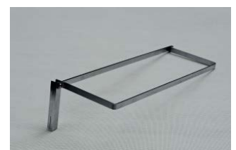
GPM ◀ 204 Sight plane (according to Schlaginhaufen) for cubic craniophor
