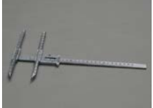
GPM ◀ 115 Coordinate caliper range: 20 -220 mm
