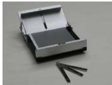
GPM ◀114 Sliding caliper (Poech type) for determining absolute and projected facial
