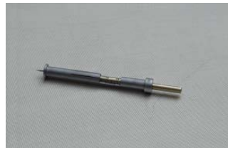
GPM ◀ 119 Skin thickness measuring instrument length: 0 –30 mm
