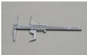
GPM ◀ 105 Sliding caliper with vernier (1/10 mm) special sliding caliper for small measurements; length: 0 – 150 mm
