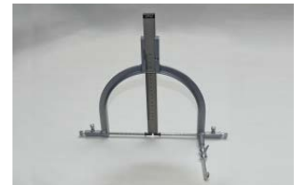
GPM ◀ 122 TODD Head spanner measuring range: 200 mm
