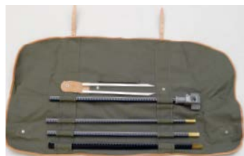
GPM ◀ 101 Anthropometer in canvas bag length: 0 – 2100 mm (0 – 950 mm) to locate measurements throughout the entire body
