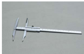
GPM ◀ 104 Sliding caliper (Martin type) length: 0 – 200 mm; depth: 0 – 50 mm
