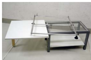
GPM ◀ 212 Rectangular diopetrograph (Martin type)
