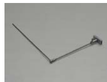
GPM ◀ 1116 Coordinate caliper (Aichel type) measuring range: 20 -300 mm
