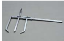
GPM ◀114 Sliding caliper (Poech type) for determining absolute and projected facial
