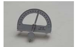
GPM ◀103 Auricular height needle for anthropometer No. 101, for measuring the auricular height of the head
