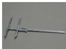
GPM ◀115 Coordinate caliper range: 20-220 mm
