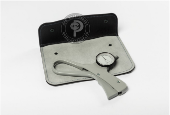
6100 «GPM» Skinfold Caliper (made in CH) to assess the degree of fatness Measuring range: 0 - 45 mm
